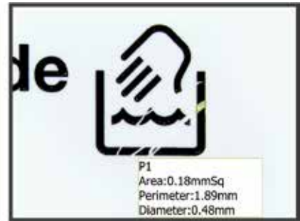
Scratch gauging on an appliance
