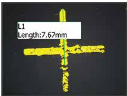
Dimensional check on a surface
